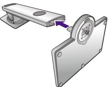
Tighten the thumbscrew on the bottom of the monitor base as illustrated.
