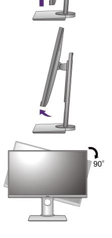
To avoid the edge of the LCD display hitting the monitor base surface while it is being rotated, do tilt and extend the monitor to the highest position before you start to rotate the display. You should also make sure there are no obstacles around the monitor and there is enough room for cables. Remove the connected USB peripherals and audio cable first.
