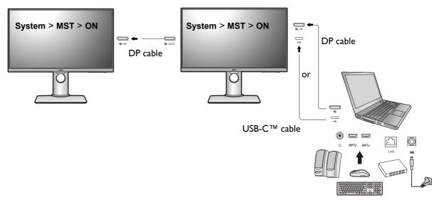
Connect your laptop to the USB-C<sup>™</sup> / DP port on the monitor using a USB-C<sup>™</sup> / DP cable. Select **Yes** to enable USB-C<sup>™</sup> power delivery in monitor standby mode if you are prompted to. The USB-C<sup>™</sup> port supplies power to the laptop then even when the monitor is in standby mode.
